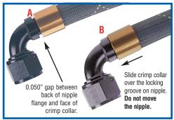
**3** Push the nipple into the hose until the back of the nipple's locking flange is approximately 0.050" away from the face of the crimp collar, as shown at **A**. Without moving the nipple, carefully slide the crimp collar over the nipple until the collar's locking flange engages the locking groove on the nipple, as shown in **B**.
