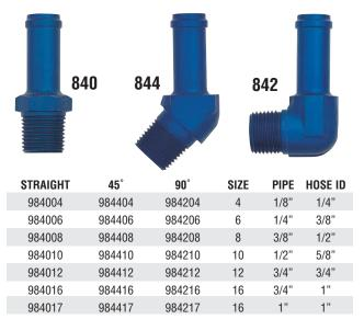
850 SERIES ALUMINUM PIPE TO TUBE ADAPTERS FOR STAINLESS STEEL RACE HOSE OR XR-31 HOSE
