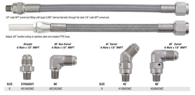
These special-made fittings were designed with a large 0.260" internal diameter hole through the 1/8" male NPT end for increased flow. The one-piece fittings are manufactured entirely from steel, while the swivel fittings have a steel body with a 1/8" male NPT thread and an aluminum forged swivel -6 nose. FOR OFF ROAD USE ONLY. DOES NOT MEET ANY D.O.T. SPECIFICATIONS.
