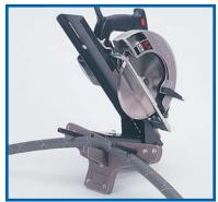
Use the XRP Hose Cut-Off Blade to cut the hose to the proper length. The toothless knife edge wheel will provide a clean and square cut. May be used on stainless steel braided hose also.
