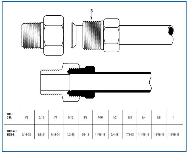
This chart shows the common thread sizes for inverted flare fittings and tubing.
