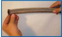
$2^{\mbox{Mark}}$  length and cut the ends with this snips.
