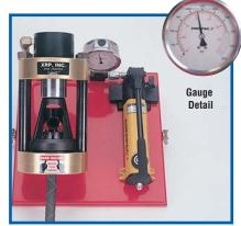
Ocontinue pumping the handle until the crimp die cage is completely closed and the pressure on the gauge indicates 4,000 to 5,000 psi. Larger sizes may require more pressure. Each die has been manufactured to provide the proper finished diameter crimp. Pressure test and inspect the finished hose assembly.
