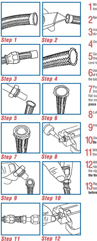
Wrap hose with tape at cut-off point and cut through the tape with a finetooth hacksaw or XRP Cut-Off Blade. **Make a clean, straight cut.**
