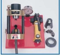
5 Position the hose assembly into the crimp die. Be careful not to disturb the nipple and collar placement.
