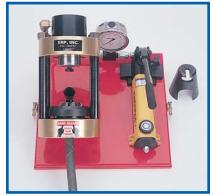
**7** Install the tapered die pusher ring plate over the crimp die. Push the plate down by hand, until the crimp die is snug on the crimp collar. Make sure the die covers the entire length of the collar.
