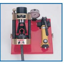
Place the pusher cone into the crimp machine and pump the handle until the cone just contacts the pusher ring plate. Now, recheck! Make certain that the crimp collar is fully covered by the crimp die and the nipple has not moved.
