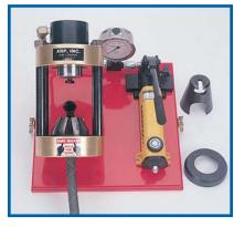
6 Place the upper half of the crimp die over the assembly in the crimper.
