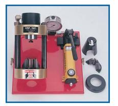
4 Insert the lower half of the crimp die into the crimping machine, making sure it is placed under the spring steel clips to hold it in place.
