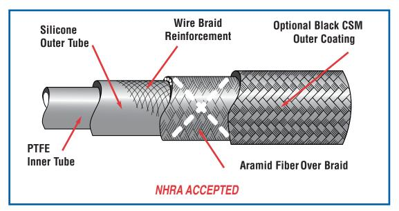
HS-79 ultra lightweight, flexible, smooth-bore PTFE hose has a 4-ply composite construction: a PTFE inner liner, Silicone outer liner, high tensile stainless steel reinforcing braid and outer braid of aramid fiber. HS-79 hose is available with a CSM outer covering as a fifth layer for added resistance against abrasion and ease of cleaning. **Features and benefits include:**
