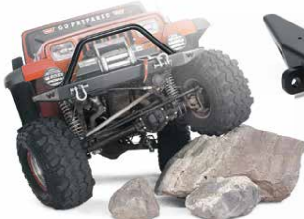
YJ WRANGLER with Front Rock Crawler Bumper, grille guard tube, and winch mounting plate
