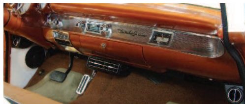
1957 Chevy installation with center plenum.
