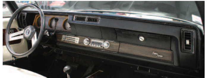
Cutlass factory-air dash with SureFit kit. (Note: SureFit installations in factory-air equipped cars use the original in-dash A/C louvers.)
