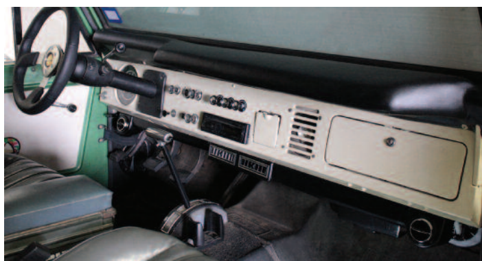
Ford Bronco dash with SureFit system with full width plenum, controls and Vintage Air louvers. 4-vent kit also available.
