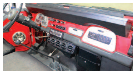
U.S. spec Toyota FJ-40 Land Cruiser dash using factory controls and Vintage Air louvers.
