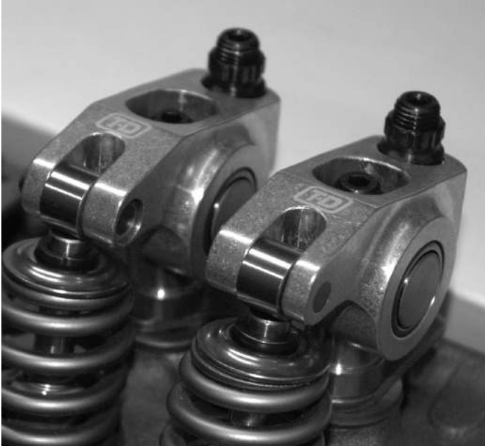
Pictured is the set-up for a small block Chevy – other stud-mount Stock Eliminator systems will differ slightly in shape to fit each individual application.
