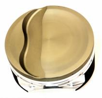
of micro-welding and provides thermal protection to the rings. We went with lateral gas ports to enhance ring sealing and not be acceptable to getting plugged like vertical gas ports. The *skirts are coated* with *Line2Line.* This process was developed by the OEM's and gives a more stabilized piston operation which is critical with large stroke engines and better ring sealing. This reduced wear again gives longer life to the engine.
