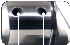
STRAIGHT SHOT & CHAMFERED OIL HOLES
