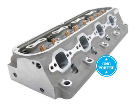
Designed with the Small Block Ford racing enthusiast in mind, these heads give you all of the benefits of professional CNC-porting – straight from the factory! However, the CNC-porting is done off of a known port, providing more airflow consistency than hand-ported runners. In addition to the CNC-ported intake and exhaust runners, the combustion chambers are also CNC-ported to moderate valve shrouding and maximize airflow efficiency.
