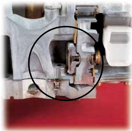
Cut-away of power valve blow-out protection.
