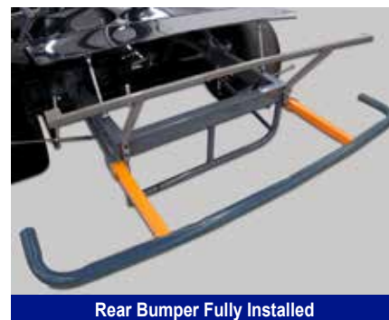
Rear Bumper Fully Installed
