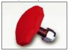
9.9158 Universal octagon bump stop. This bump stop measures 1 7/8" across from flat side to flat side, 1 1/16" tall, 2" dia. 2 per set.
