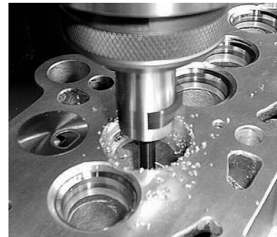
Picture 5 - Cutting the counter bore
