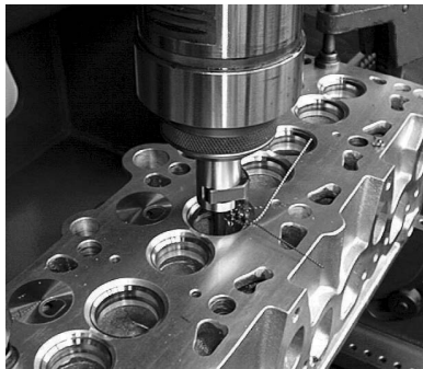
Picture 3 - Cutting valve seat inserts
