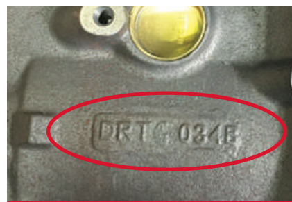
MRK IV, Gen V and Gen VI blocks with water between the bores are identified by a B suffix on the casting number.
