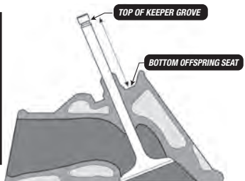
Diagram 1. Calculating Installed Spring Height
