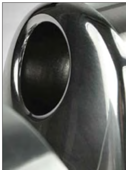
Rod journal holes and main bearing gun drill bores are all highly polished and radiused.
