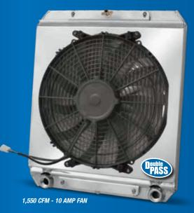
AFCO's Double pass "Dragster" radiator is specifically designed for roadsters and dragsters. It features a 16 fin per inch, no epoxy core for maximum efficiency, as well as a high CFM / low AMP draw fan & shroud combo. This radiator comes complete with a fan on/off switch, 4 mounting bosses and 3/4" FNPT (Female National Pipe Thread) inlet/outlet.
