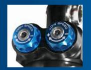
HIGH SPEED COMPRESSION ADJUSTMENT. LOW SPEED COMPRESSION ADJUSTMENT.
