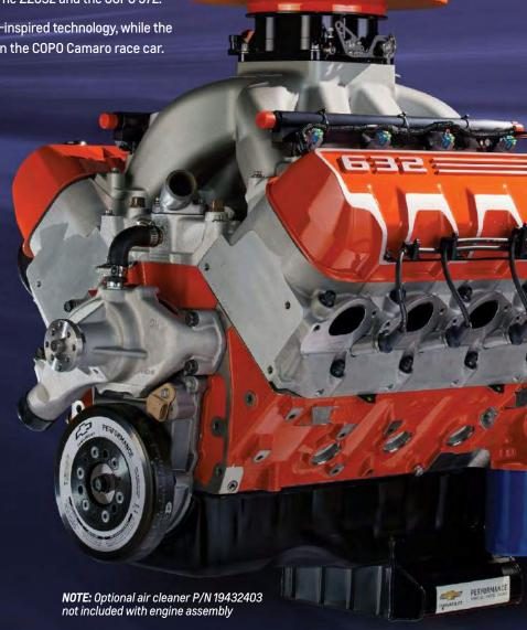
The new raised runner and parallel-port RS-X heads were inspired by the straight-flow design of Pro Stock heads that have their roots in the famed "DRCE" racing engine. They have enormous 449cc intake runners that support 481 cfm of airfow at .787-in. lift. In short, they flow huge! And they support a 7,000-rpm capability for the ZZ632.
