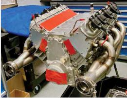
Left: This is what 1,000 turbocharged horsepower looks like with an LS9 long block, an LS3 intake manifold, twin turbos and an E85 fuel system.
