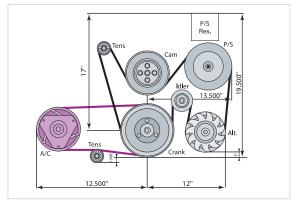
CTS-V Accessory Drive System – with A/C, Fixed Displacement Compressor
