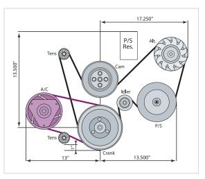
Corvette Accessory Drive System - with A/C
