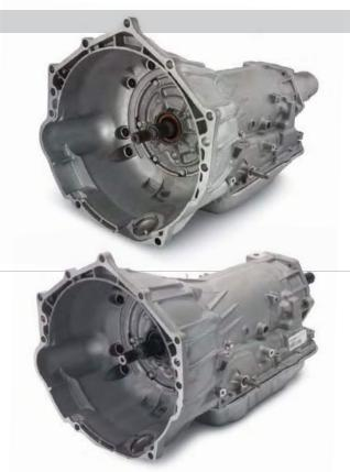
**NOTE:** Use with electronic controller P/N 19332775 for carbureted and Ram Jet applications. Use with electronic controller P/N 19302405 with Chevrolet Performance LS and LT fuel-injected applications.
