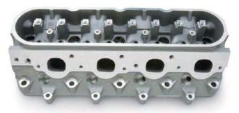
LSX-LS7 Cylinder Head Assembly (exhaust)
