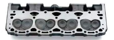
Cast-Iron Vortec Cylinder Head (combustion chamber)
