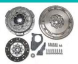
Transmission Installation Kit - TREMEC TR6060 (MG9), 8-Bolt Flange
