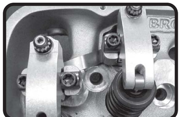
**STEP 6:** TORQUE ROCKER SHAFT BOLTS TO **26-28 LBS-FT** AND SET VALVE LASH ACCORDING TO THE INSTRUCTIONS ON THE REVERSE SIDE. LUBRICATE ROCKERS WITH ENGINE OIL. ROTATE ENGINE 90-DEGREES AND REPEAT STEPS FIVE AND SIX TO REMAINING CYLINDERS FOLLOWING ENGINE FIRING ORDER (**18436572**).
