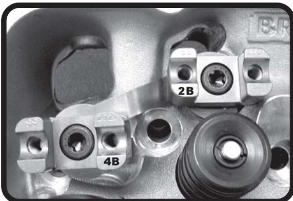
**STEP 3:** APPLY OIL TO 7/16 X 1" STAND BOLT AND BOLT THE **2021-4B** STAND TO EXHAUST STUD BOSS. MAKE SURE BOTH STANDS ARE FULLY ENGAGED IN THE STAND LINKS™. TORQUE BOTH THE INTAKE AND EXHAUST STAND BOLTS TO **60-65 LBS-FT.** REPEAT STEPS TWO AND THREE ON REMAINING CYLINDERS.
