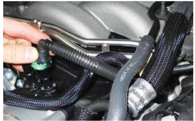
EECPV tube quick connector with green lock
