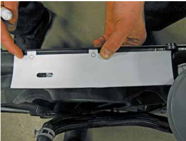
Proper template position on fan shroud
