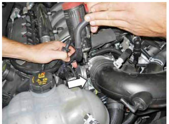
Clamp at throttle body
