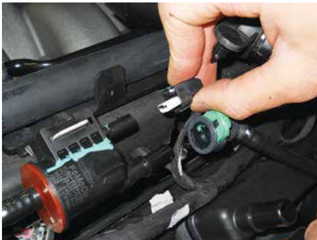
EECPV electrical connector
