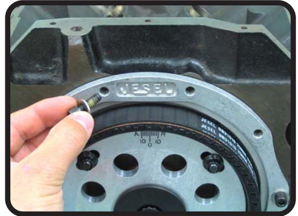
**STEP 1:** WHEN INSTALLING THE JESEL DISTRIBUTOR DRIVE ON AN ENGINE ALREADY EQUIPPED WITH A JESEL BELT DRIVE SYSTEM, BEGIN BY REMOVING THE TOP FOUR COVER BOLTS FROM THE BLOCK. WITH THE COVER BOLTS REMOVED, LOOSEN AND REMOVE THE **CENTER LH THREAD** CAM BOLT AND REMOVE THE CAMSHAFT ADAPTER WASHER FROM THE FRONT OF THE ENGINE. THERE IS AN INSTRUCTION SHEET INCLUDED WITH ALL JESEL BELT DRIVE SYSTEMS IF YOU ARE INSTALLING BOTH KITS AT THE SAME TIME.
